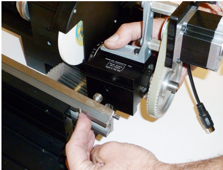
Fig. 14—Slide the headstock onto the pin while pushing the pin into place with the other hand.
