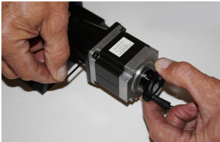
Fig. 6. Secure the set screw to lock motor shaft into the coupling.
