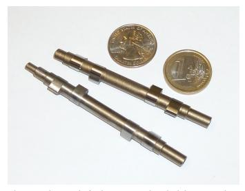
These are the camshafts that were produced while writing these instructions; however, the shaft ends haven't been ground to size yet.
