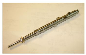
The finished camshaft for a four cylinder inline Seal Engine
