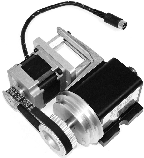
Figure 1—Alternate stepper location. By mounting the motor bracket in the opposite direction on the headstock, the motor will turn the spindle in the same direction as the stepper motor is turning. It also saves a little space if that is a consideration in your particular application.
